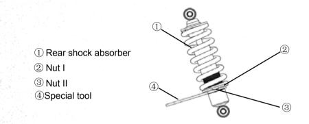
WARNING This unit contains high pressure nitrogen gas. Mis-handling can cause explosion. Do not incinerate, puncture or open it.
