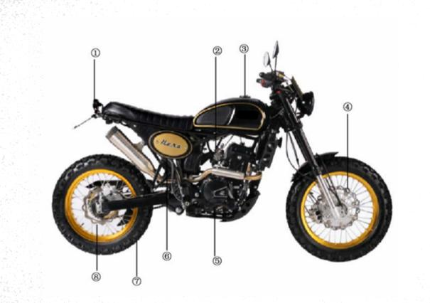
Rear light, ② Throttle valve , ③ Cap,fuel tank, ④ Front brake disc, ⑤ Rear brake pedal,
