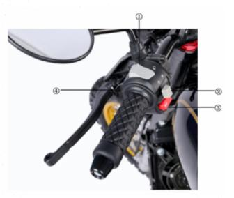
(1)Dimmer switch (2)Turn light switch (3)Horn button (4)Override light switch
