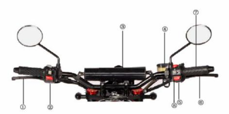
①Clutch lever ②Handlebar switches, LH ③Meter instruments ④Front brake fluid reservoir
