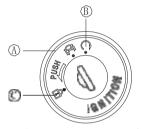
A Off B On C Steering Locked
