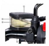
① Front brake fluid cap ② Upper level line ③ Lower level line ④ Front brake fluid reservoir
