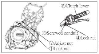
Figure 19 Clutch Cable Inspection
