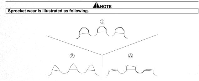
① Standard Teeth ② Wear Teeth ③ Damaged Teeth
