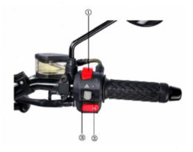
①Engine stop switch ②Light switch ③Warning button
