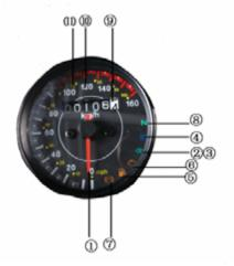
①Tachometer ②Turn indicator, LH ③Turn indicator, RH ④High-beam indicator ⑤Fuel diaplay
