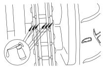
If the chain is especially dry, clean it before lubrication.
